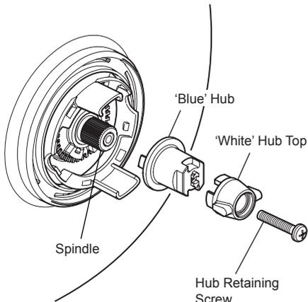
6. Once the desired maximum blend temperature has been achieved, refit the 'blue' hub without disturbing the spindle.
