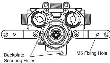
5. Drill the two 5.5 mm holes for the fixing positions (countersink the holes at the front).
