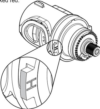
**Note!** Should the supplies be reversed then the mixing valve will not be able to control temperature. This can be corrected by rotating the thermostatic cartridge within the valve body, refer to section: **'Installation, Outlet Position/ Reversed Inlet Supplies'**.
