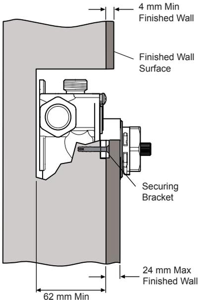
3. Fit the securing brackets to the mixer with the bracket securing screws.
