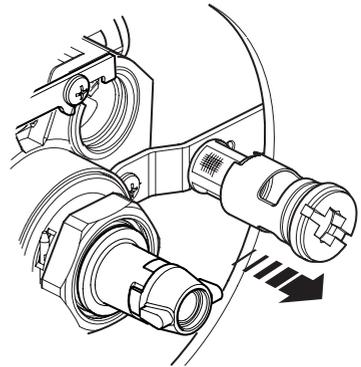
7. The non return valve assembly and/or strainer screens can be cleaned or replaced as necessary.
