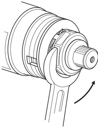
4. Remove the indicator trim (adjustable models) and pull the thermostatic cartridge free of the valve body.
