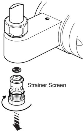
3. The non return valve cartridge and/or strainer screens can be cleaned or replaced as necessary.
