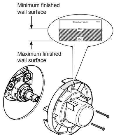
18. Remove the two shroud screws (retain for later use) and remove the building-in shroud.
