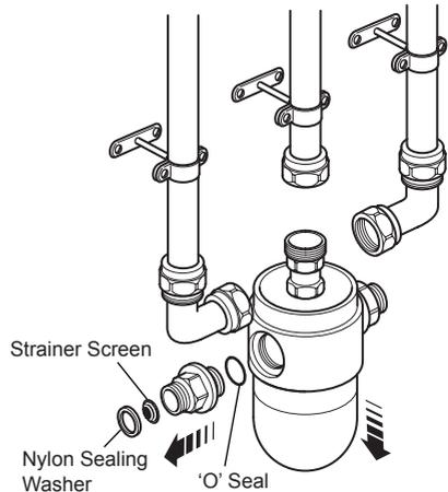
4. The non return valve cartridge and/or strainer screens can be cleaned or replaced as necessary.
