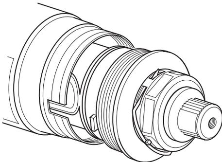
7. Carefully align and then tighten the head nut, do not over-tighten (max torque 2.5 N/m - 1.85 lbf ft).
