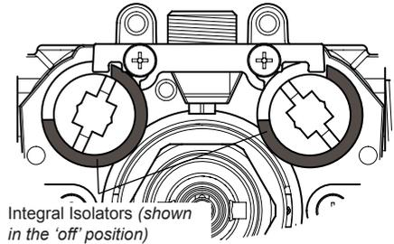
5. Open an outlet fitting to release pressure and to assist the draining of residual water.
