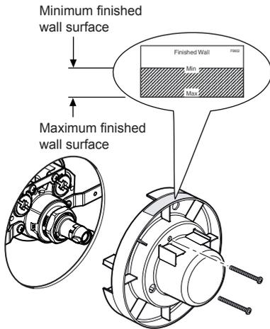
15. Remove the two shroud screws (retain for later use) and remove the building-in shroud.
