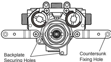
4. Make sure that the mixer is level and mark the positions for the countersunk fixing holes on the wall.
