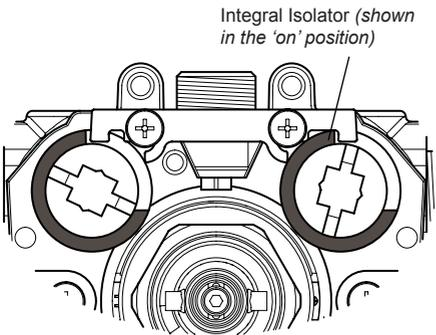
12. Align the slots in the 'black' knob retainer with the lugs on the 'white' hub top and secure the backplate to the mixing valve with the two backplate screws.
