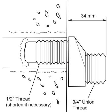
3. Screw pipe concealing plates onto offset connectors.
