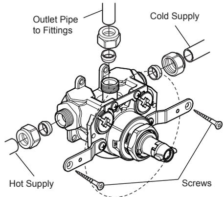
12. Turn on the water supplies and check for leaks.
