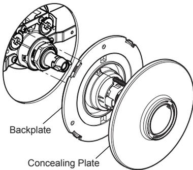
4. Using a 10 mm hexagonal key turn the integral isolators 90° anti-clockwise to shut off the hot and cold water supplies.
