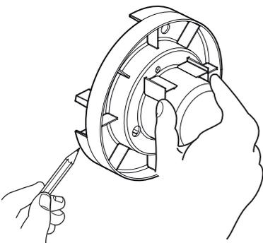
4. Mark the routes for the hot and cold supply pipework (**Hot - Left, Cold - Right**) and for the outlet pipework.
